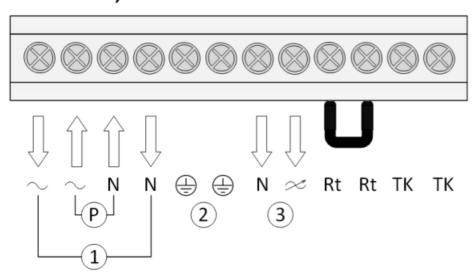
Transmisson:between  $\sim$  and N is always 230V when the transformer handle is in pos. 1-5
