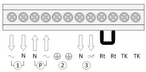
Transmisson:between  $^{\sim}$  and N is always 230V when the transformer handle is in pos. 1-5
