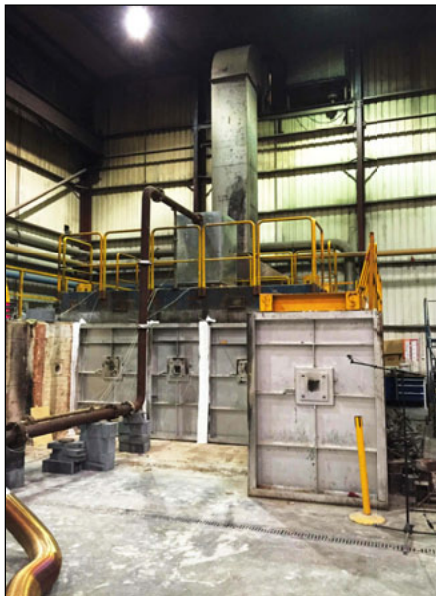
Fire testing rig for the testing of horizontally mounted dampers.
