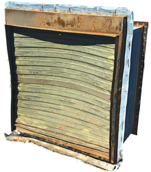
Series 100 fire damper c/w plate frame after a successful fire test
